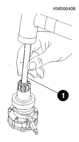
Disassembling overrunning-clutch drive
